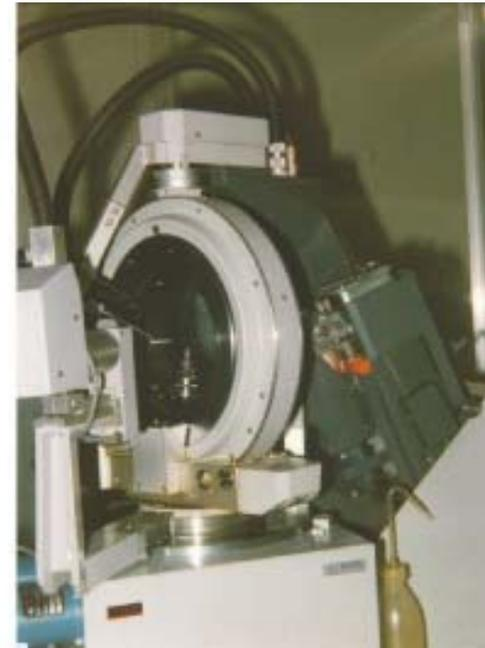
In the case of kappa geometry the  $\chi$  circle is made up of two other angles  $\kappa$  and  $\omega_{\kappa}$
